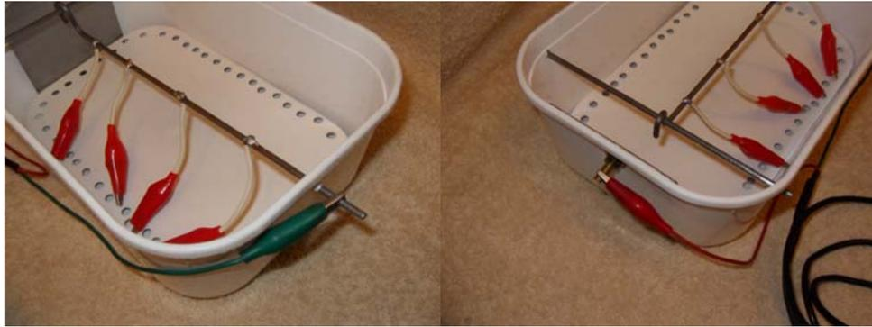
As can be seen in the above photos. The negative terminal is connected to the clip bar, and the positive terminal to the electrode plate. Do not switch these two wires around, as you will be doing electroplating. The easiest way to see if they are connected properly is when you switch it on, the artifact will bubble.... If the plate bubbles, switch the wires around.
