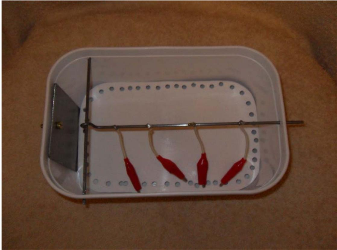
As can be seen from the photo above, the rod goes through the plastic at the end of the container so that the negative terminal of the power supply has something to hold onto.
