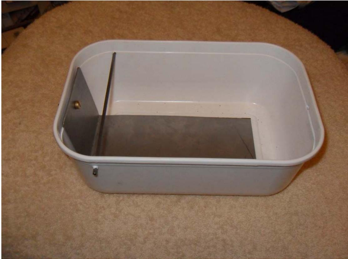
What I have done is to cut and bend the stainless steel plate to fit nicely into the ice cream container. I have attached the plate to the container using a 5mm brass bolt, this being the contact for the positive wire.
