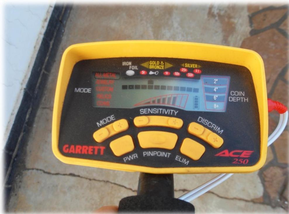
The aluminium pull-tab reading
