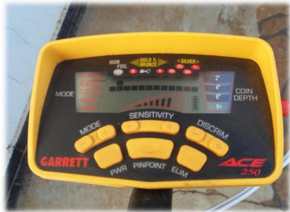
With the nail on top of the coin, the reading is showing iron on the 2<sup>nd</sup> segment. The coin has disappeared which for me is a lost find. What is amazing is that the size of the Penny is just under 1 ¼ inches in diameter / 30mm which is a large object which is lost. With the objects switched around, the Penny is the most dominant item shown
